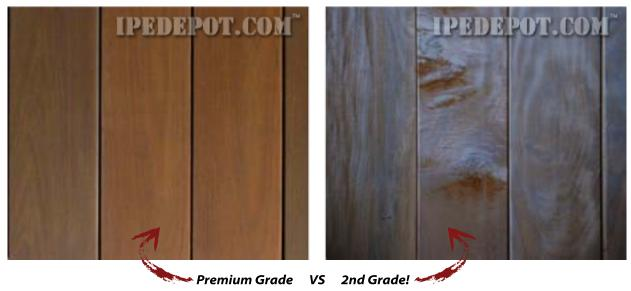
As you can see, Premium grade lpe does not have the visible defects that is common in 2nd grade material. You can often find 2nd grade material a high amount of knots, and milling defects.
